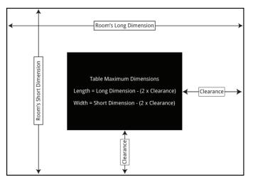
For spaces up to 16ft long, minimum clearance is 42", while 48" is recommended.
